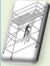
**Scaffolding** refers to the plant components and materials that, when assembled, form a scaffold.
