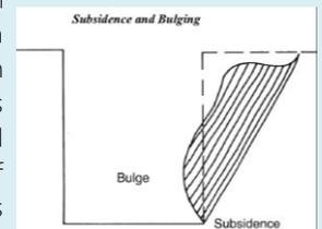
**Heaving or Squeezing** Bottom heaving or squeezing is caused by the downward pressure created by the weight of adjoining soil. This pressure causes a bulge in the bottom of the cut
