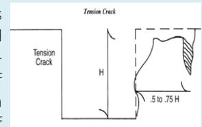
**Sliding or sluffing** may occur as a result of tension cracks,
