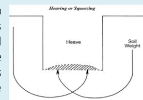
**Boiling** is evidenced by an upward water flow into the bottom of the cut. A high water table is one of the causes of boiling. Boiling produces a "quick" condition in the bottom of the cut and can occur even when shoring or trench boxes are used.
